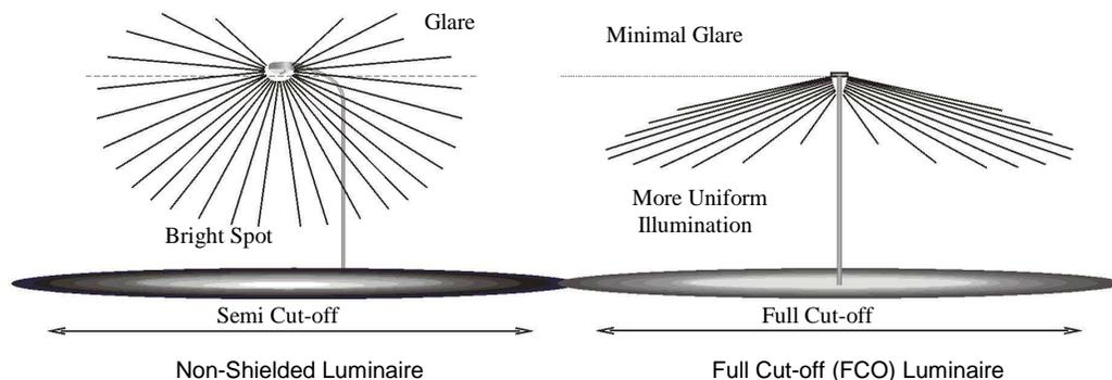
Semi Cut-off and Full Cut-off Luminaires
